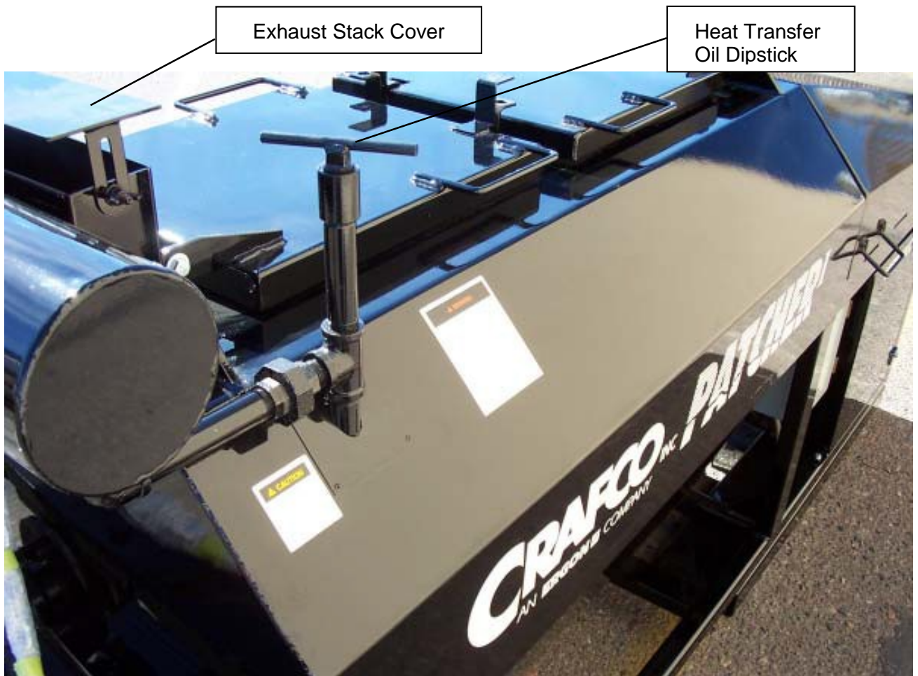
Figure 5.3 Heat Transfer Oil Dipstick
