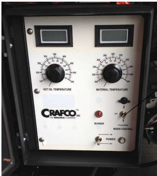
Figure 5.5 Mixer Control Switch
